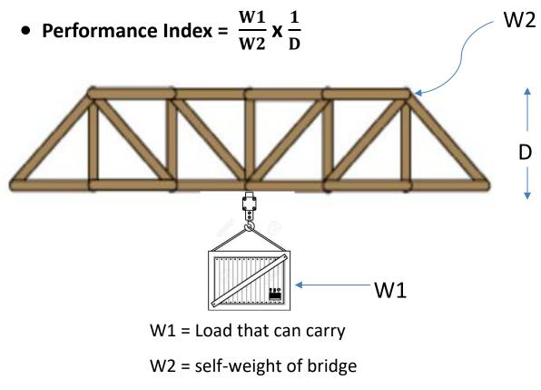
D = Depth of Bridge Span
